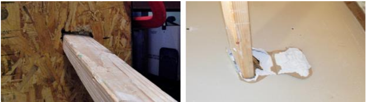
Figure 4-22: Panel M-C Typical Front (Left) and Rear (Right) Damage
