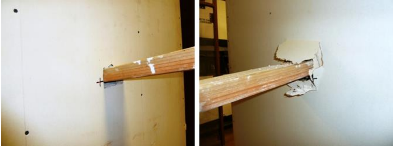
Figure 4-45: Panel 5 Typical Front (Left) and Rear (Right) Damage
