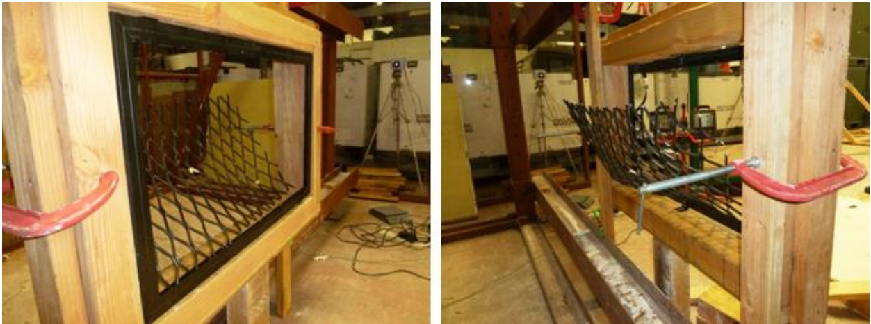
Figure 4-56: Small Window Screen Typical Front (Left) and Rear (Right) Damage
