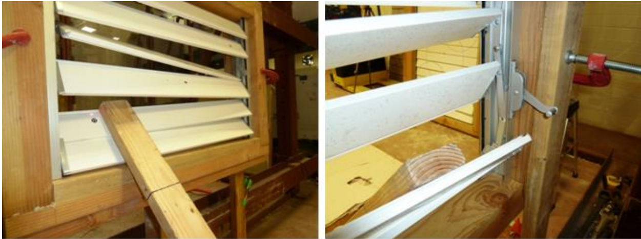
Figure 4-48: Small Louver Typical Front (Left) and Rear (Right) Damage
