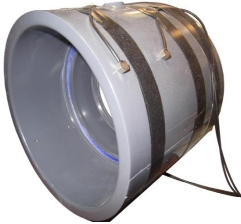
Figure 3-6: Timing Device with Installed Fiber Optic Sensors
