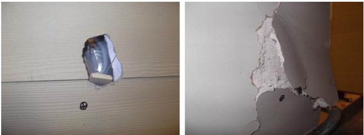
Figure 4-35: Panel 2 Typical Front (Left) and Rear (Right) Damage
