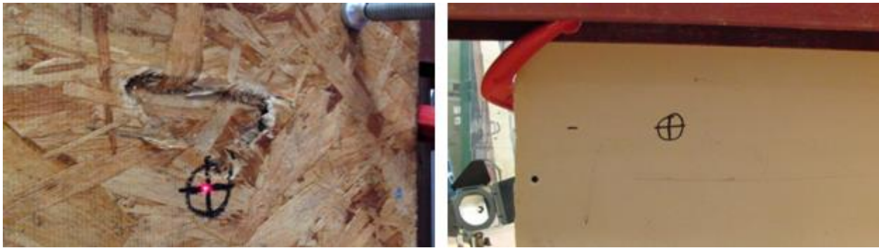
Figure 4-24: Panel M-D Typical Front (Left) and Rear (Right) Damage
