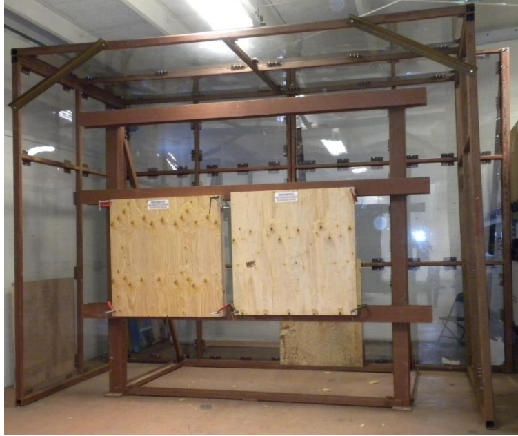
Figure 3-8: Steel Test Frame Surrounded by Polycarbonate Protection Barrier
