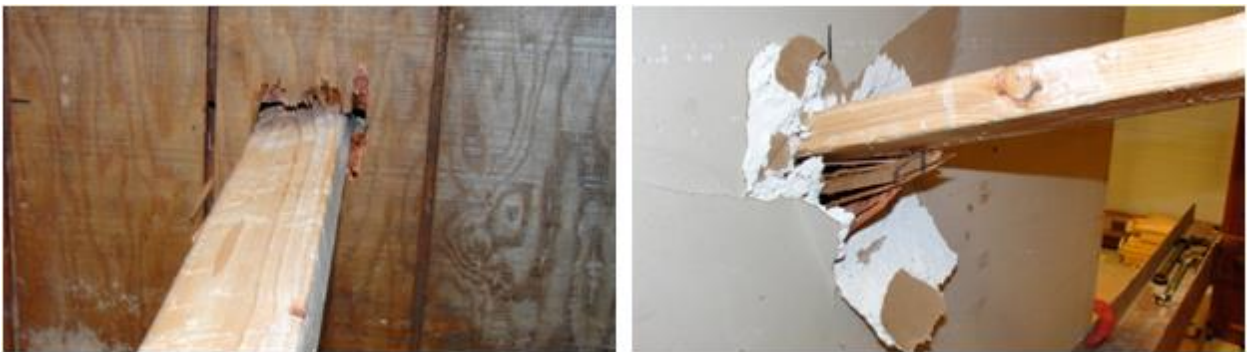
Figure 4-16: Panel Control M-O Typical Front (Left) and Rear (Right) Damage
