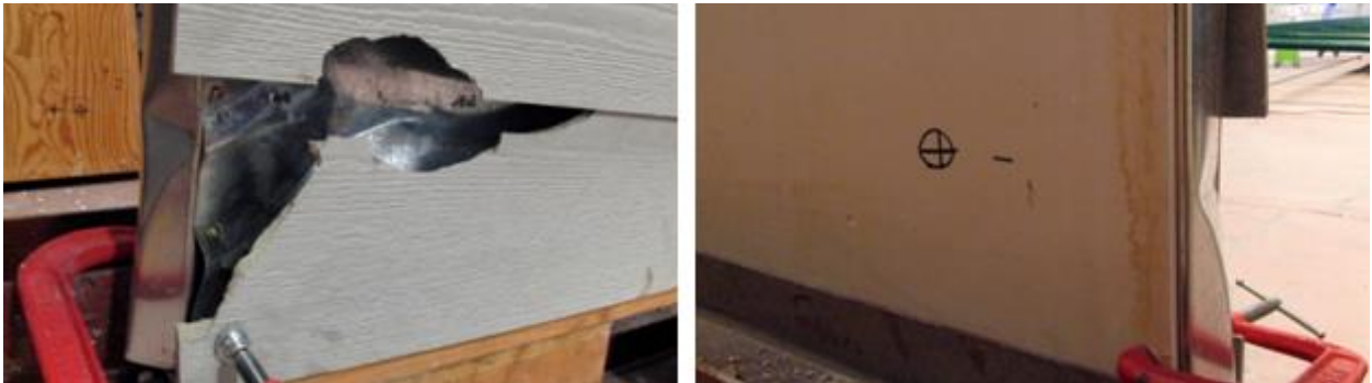
Figure 4-31: Panel M-G Typical Front (Left) and Rear (Right) Damage
