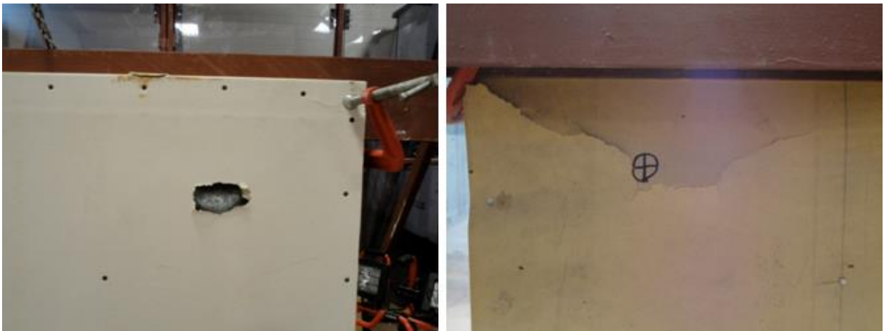
Figure 4-43: Panel 4' Typical Front (Left) and Rear (Right) Damage
