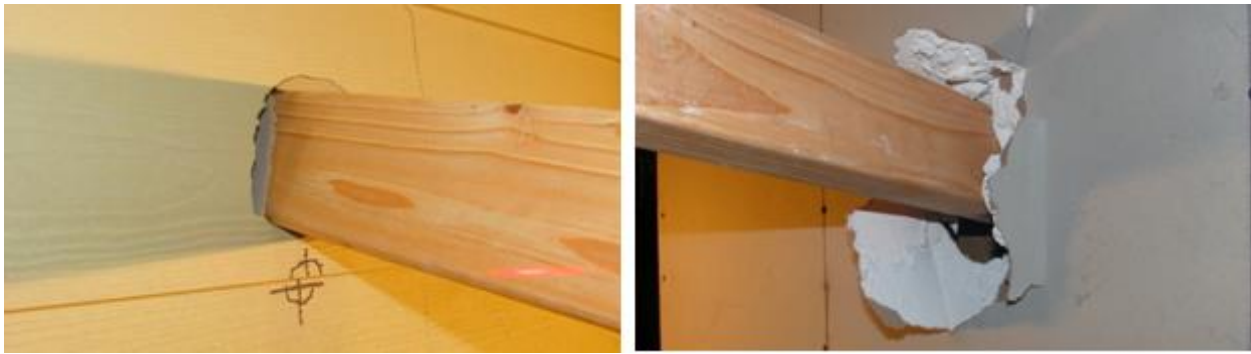
Figure 4-6: Panel B Front (Left) and Rear (Right) Damage for Bottom Left Test
