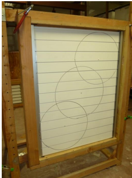
Figure 4-50: Medium Louver Sustained No Damage from Small Missiles
