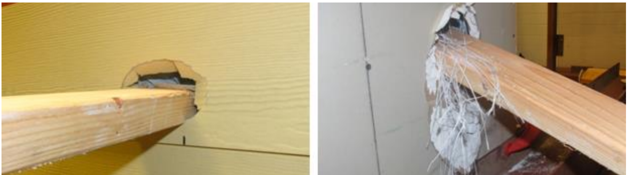
Figure 4-4: Panel A Typical Front (Left) and Rear (Right) Damage
