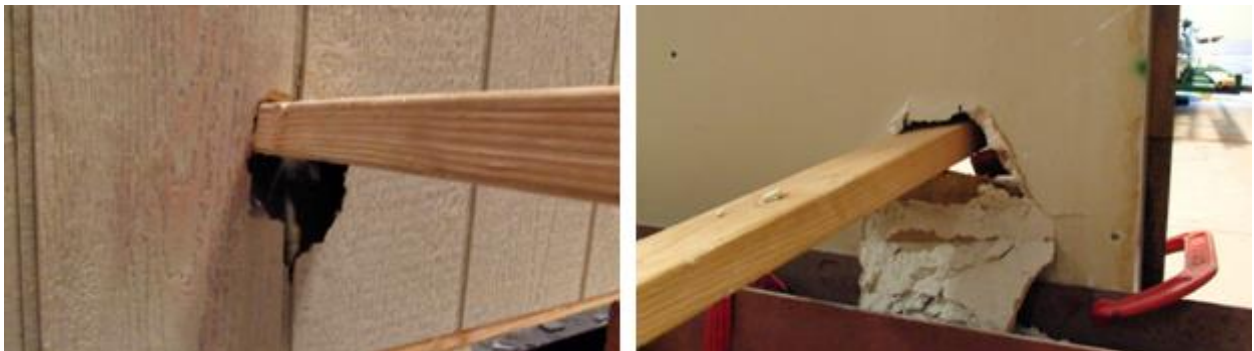
Figure 4-20: Panel M-B Typical Front (Left) and Rear (Right) Damage
