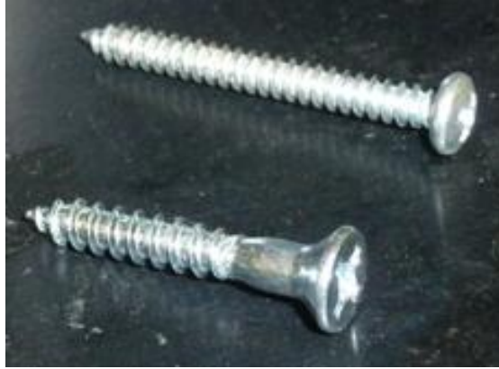
Figure 4-46: Screw Replacement for Louver Assemblies (Upper #8 screw replaced by lower #10 wood screw)
