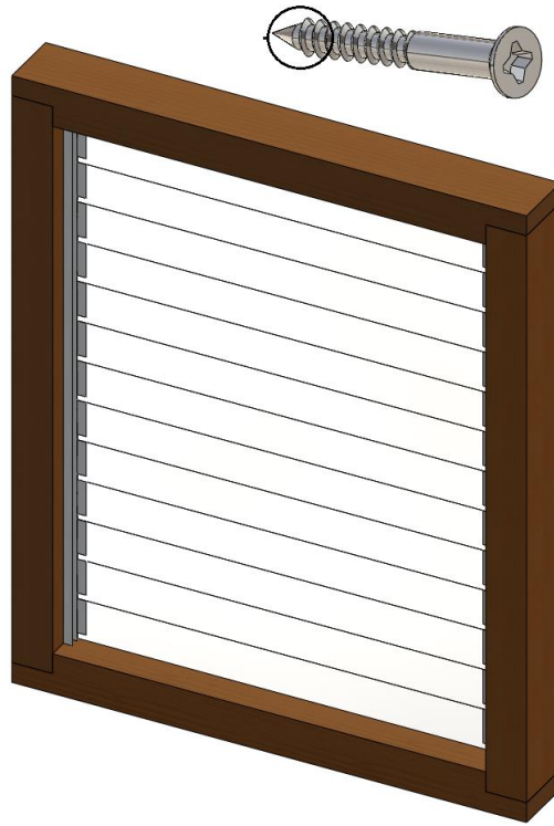
Figure 4-49: Medium Louver Fenestration Assembly
