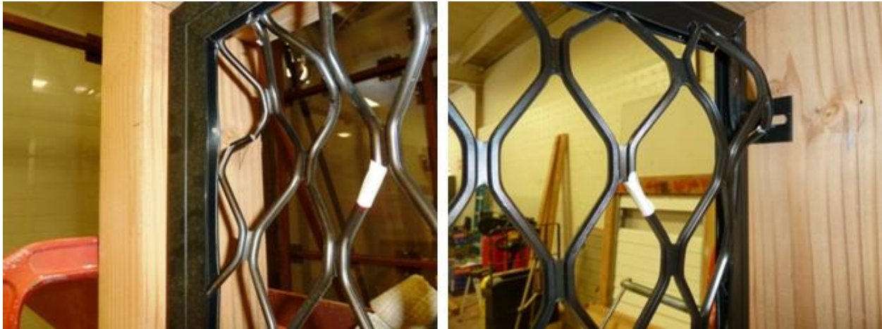
Figure 4-58: Large Window Screen Typical Front (Left) and Rear (Right) Damage
