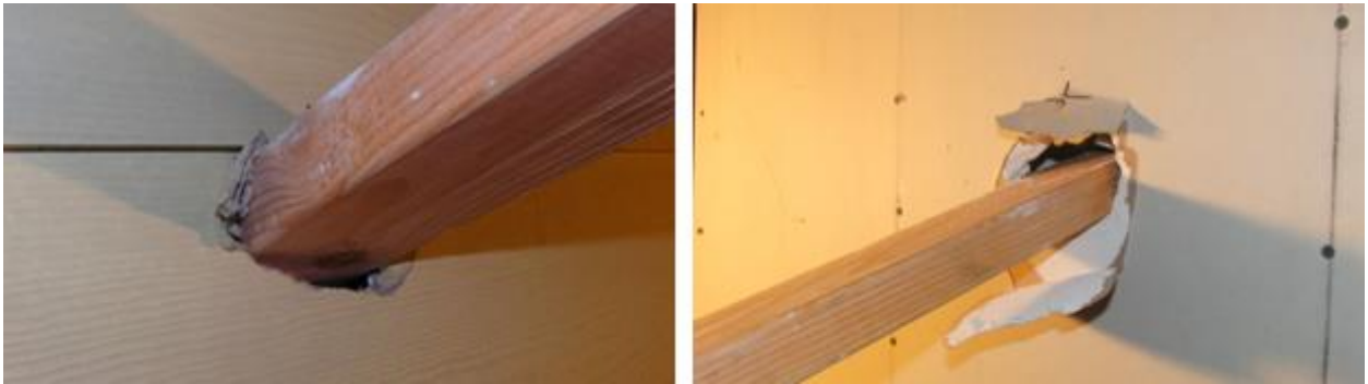
Figure 4-2: Panel O Typical Front (Left) and Rear (Right) Damage
