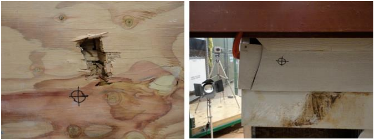
Figure 4-29: Panel M-F' Typical Front (Left) and Rear (Right) Damage
