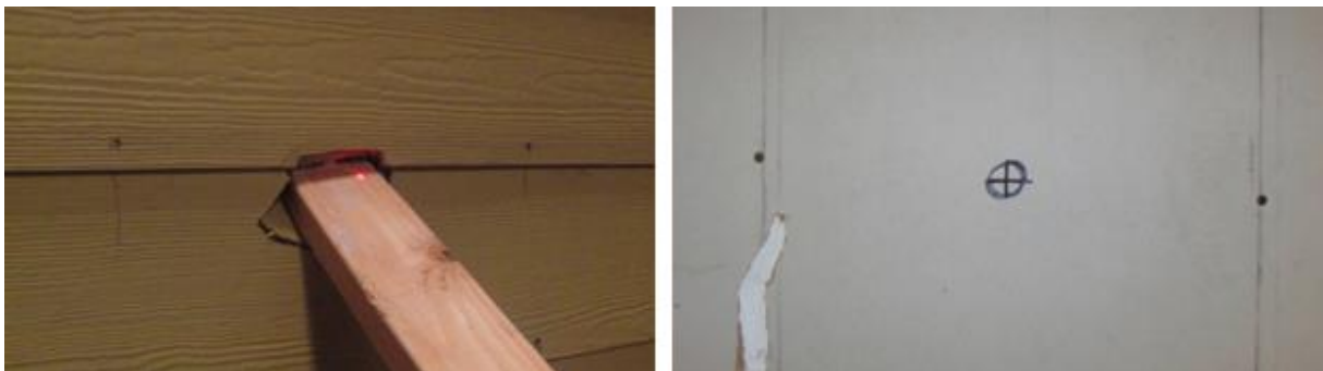
Figure 4-8: Panel C Front (Left) and Rear (Right) Damage for Three Passing Tests
