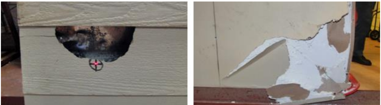
Figure 4-14: Panel H Typical Front (Left) and Rear (Right) Damage
