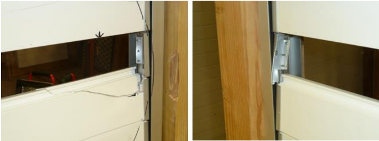
Figure 4-51: Medium Louver Typical Front (Left) and Rear (Right) Damage from Large Missile
