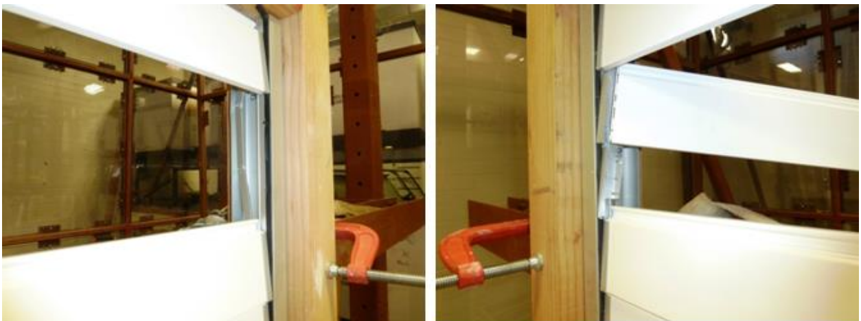
Figure 4-53: Large Louver Typical Front (Left) and Rear (Right) Damage
