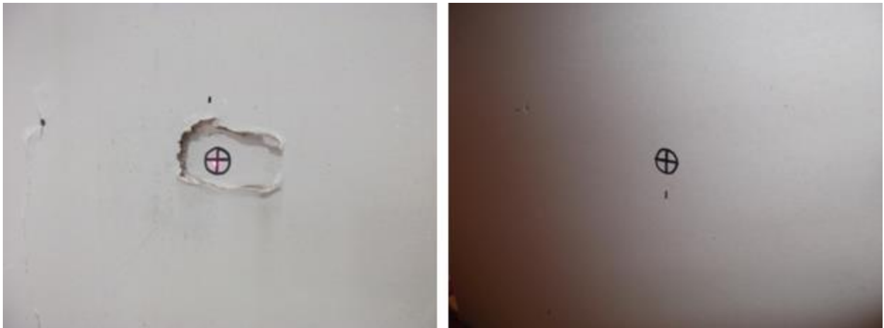
Figure 4-39: Panel 3' Typical Front (Left) and Rear (Right) Damage
