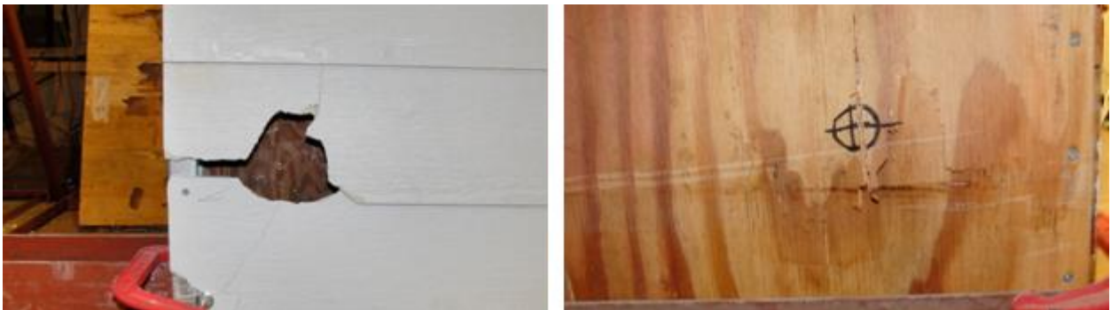
Figure 4-28: Panel M-F Front (Left) and Rear (Right) Damage for Bottom Left Test
