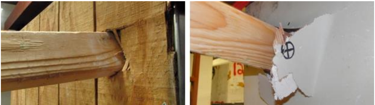
Figure 4-10: Panel O' Typical Front (Left) and Rear (Right) Damage
