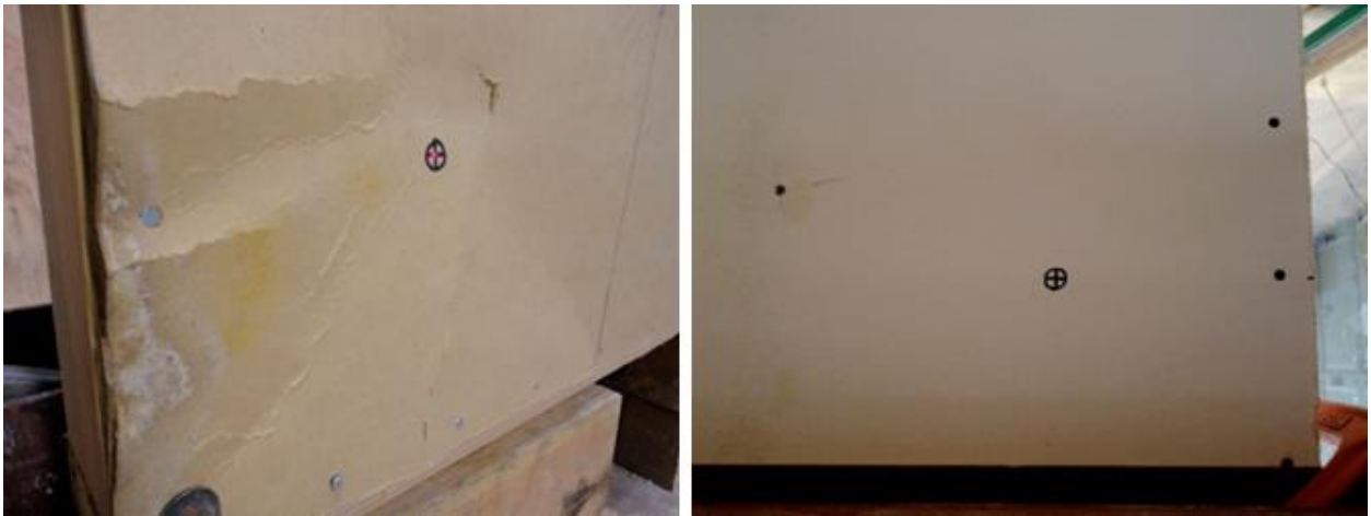
Figure 4-41: Panel 4 Typical Front (Left) and Rear (Right) Damage
