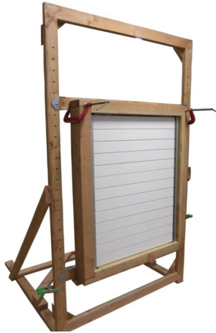
Figure 3-26: Mini Frame for Small Missile Test
