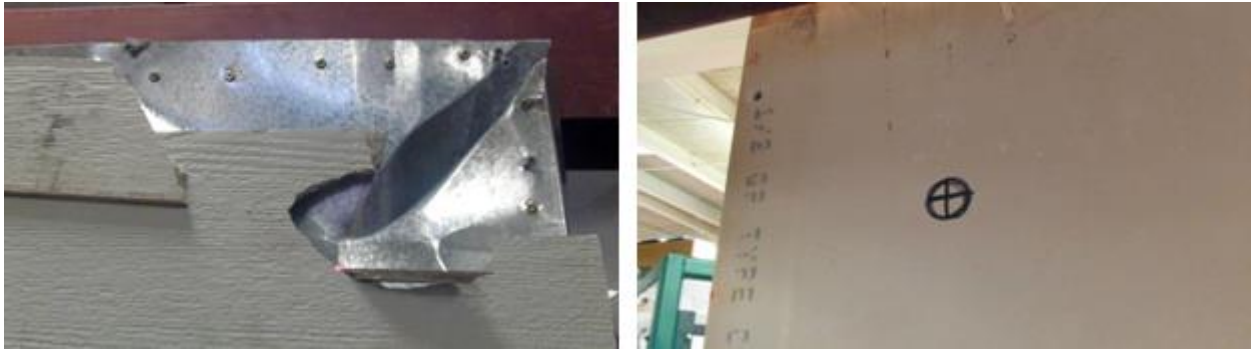
Figure 4-12: Panel G' Typical Front (Left) and Rear (Right) Damage
