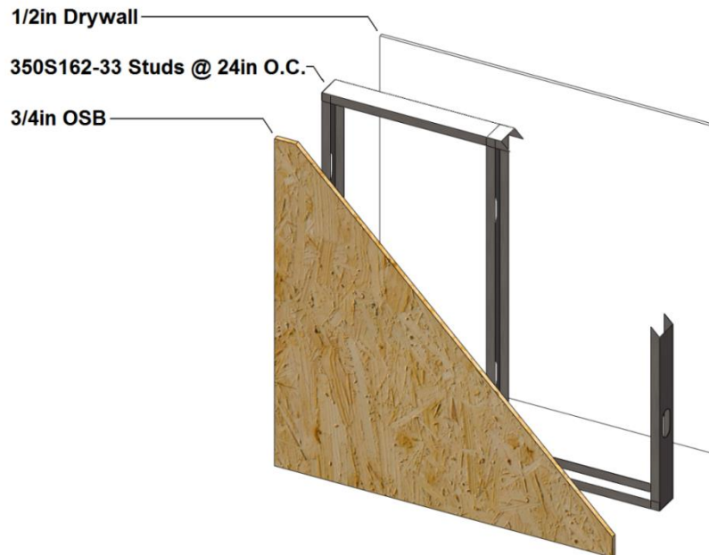
Figure 4-23: Panel M-D Exploded View
