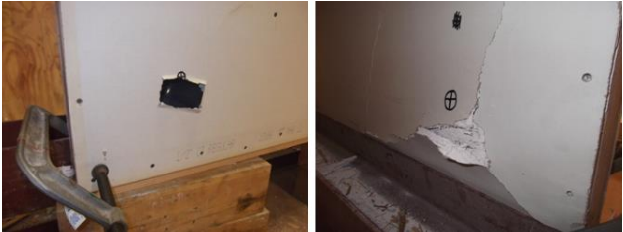
Figure 4-37: Panel 3 Typical Front (Left) and Rear (Right) Damage
