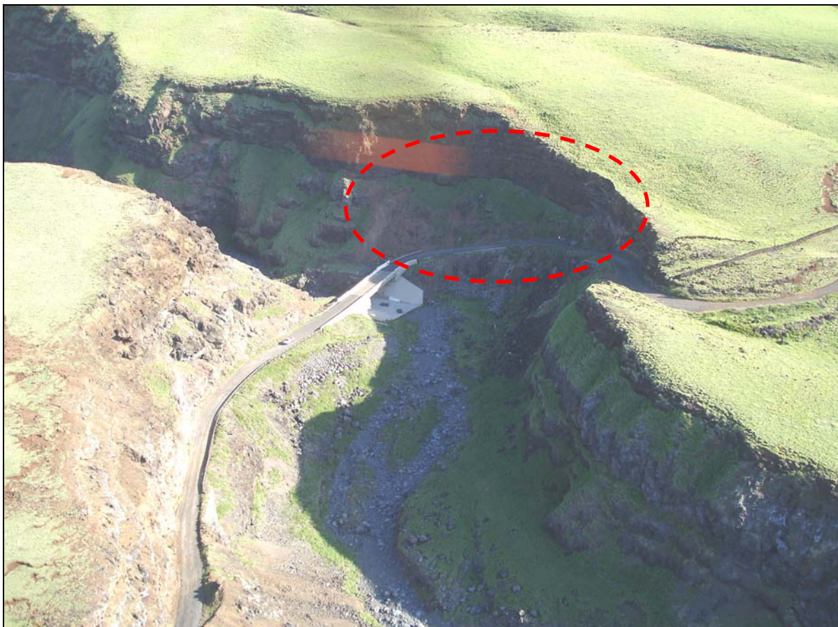
Figure 14 Manawainui, Maui (incipient rockfall over the roadway indicated on the photograph) (Photographs courtesy of Maui Civil Defense Agency)
